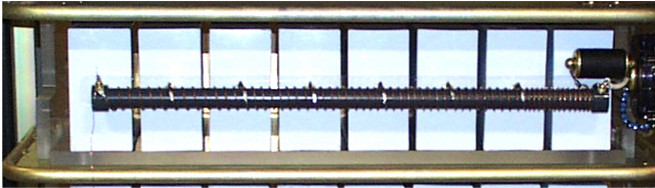
DARHT-II at LANL, 2 \mu s, tapered impedance with decreasing inductance values
